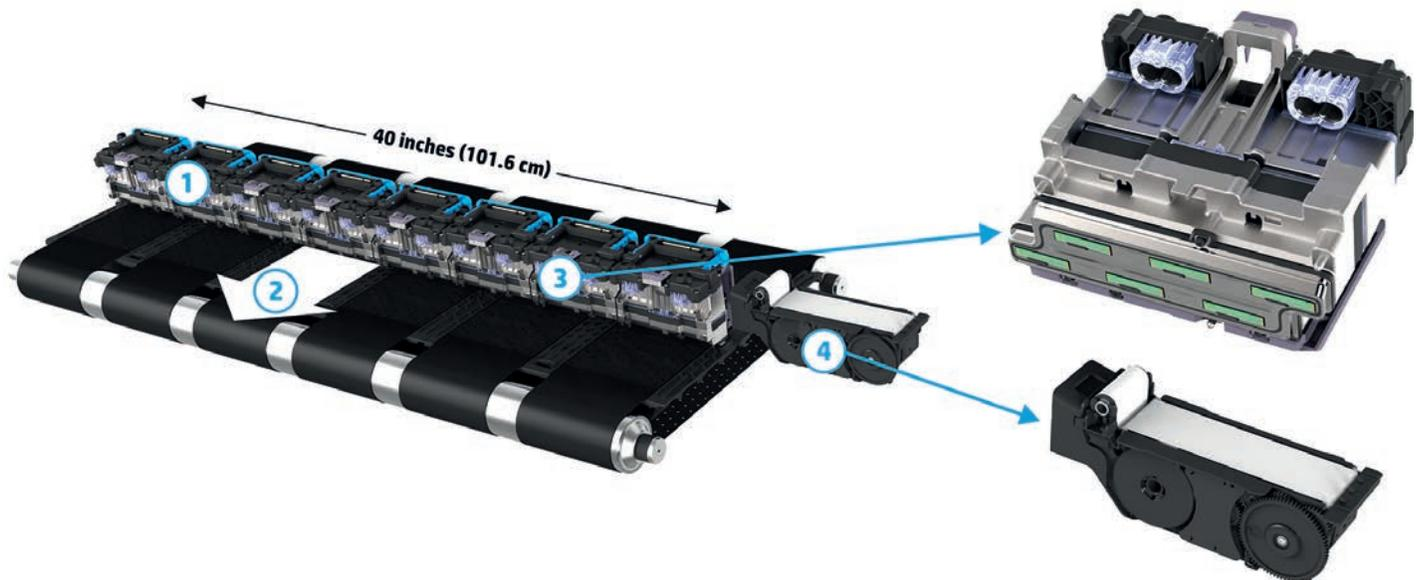
HP PageWide XL printers include a stationary 40-inch (101.6-cm) printbar **(1)** that spans the whole printing width. The entire page is printed in one pass **(2)**, enabling very high printing speeds.
